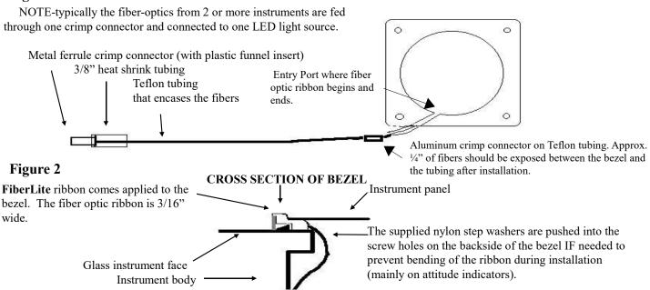
**FiberLites** are designed to sandwich between the instrument and the panel as shown in Figure 2. This will recess the instrument approximately 3/16". The bezels come in three different sizes: 2-1/4", 3-1/8" and 3-1/8" with one cutout for knobs. The bezel with the cutout can be rotated to fit either a left or right knob, but in order to keep the bright spot on top, you will need to use a dremel to cut out the bottom left corner for a bottom left knob.
