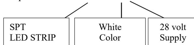
Supply voltage wiring: The RED wire is for input (+) voltage (if using the SPTPWM dimmer, the red wire connects to the YELLOW output screw terminal). Connect the BLACK wire to a secure aircraft ground.
